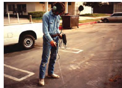
Ultrasonic detection can be used to locate underground system leaks and detect heat exchanger tube leakage.
