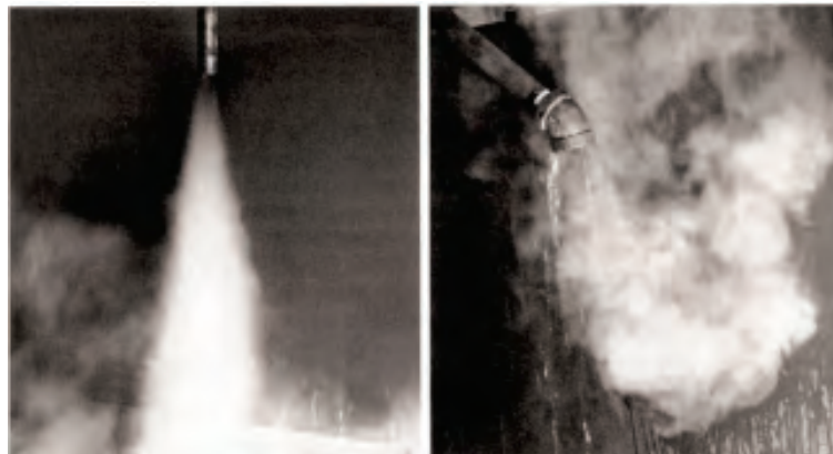
Figure 9.3.7. Live steam (left) versus flash steam (right)
