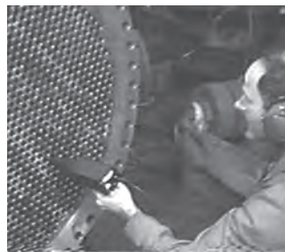
Ultrasonic detection can be used to locate underground system leaks and detect heat exchanger tube leakage.
