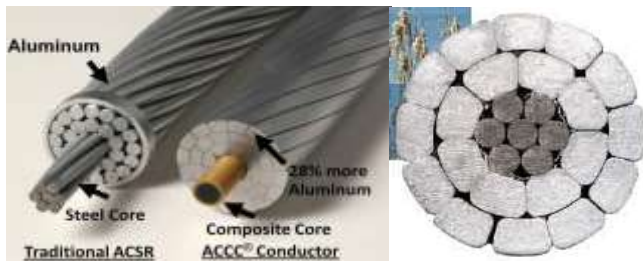
Fig.2: ACSR and ACCC conductor, Source: CEMIG, 2010
