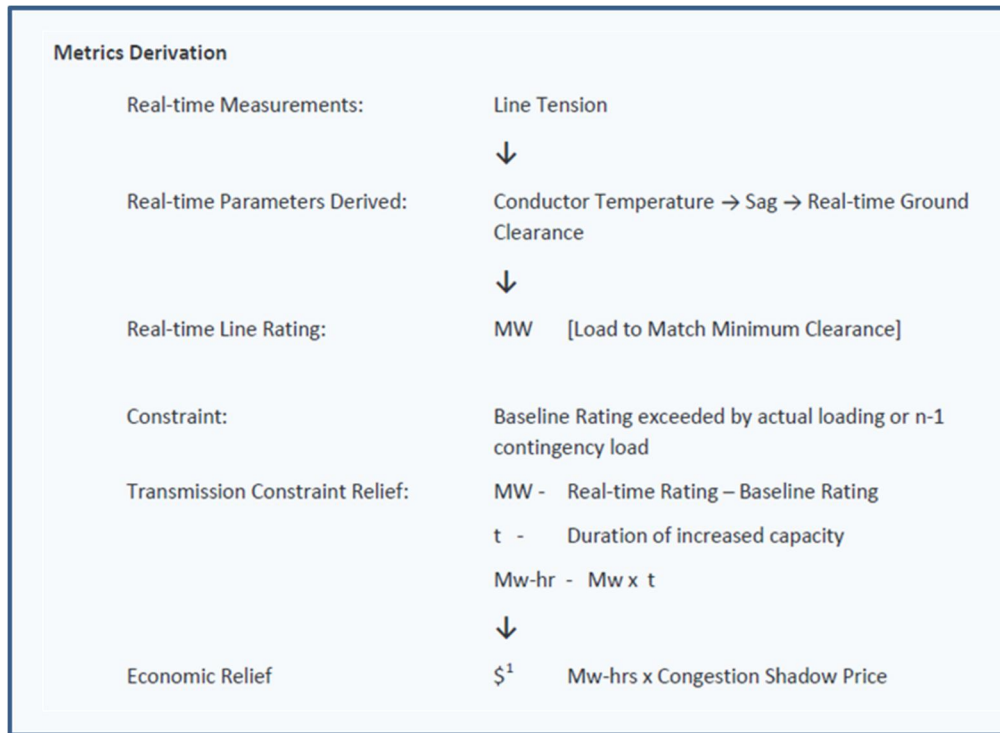
Figure 20. Metrics Derivation for various measurable quantities to define the benefits derived from dynamic line rating. [17]
